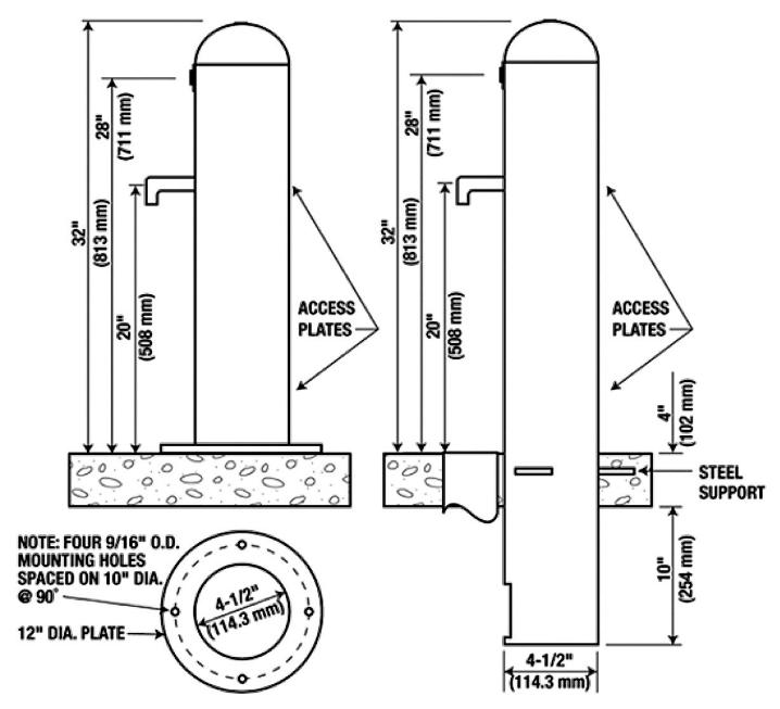
NOTE: 1) Used with inground valve system SW-PBFP (7000-34) and SNW-PBFP (7000-34-FPS)
