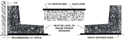
support sink or floor in case the sub floor is uneven. Grout exposed edges.
